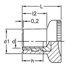
$\begin{array}{ll} D & = 31 \\ d1 & = 18.5 \\ d \ 6H = M10 \\ h & = 17 \\ L & = 27.0 \end{array}$
